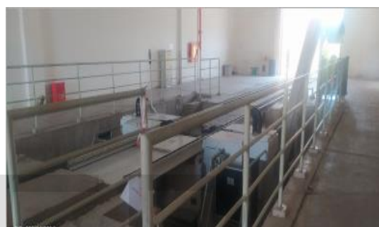
B. Under Floor wheel lathe machine at Addis Ababa Light Rail Transit Service
